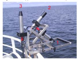
The sensor 1 measures the above water signal. The sensor 2 measures the atmospheric signal. The reflection law is applied to the measurement 2 to subtract to measurement 1 the sky dome reflection. The sensor 3 measures the total solar energy.
